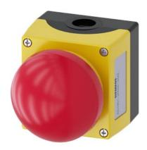
Enclosure for command devices, 22 mm, round, Enclosure material plastic, Enclosure top part yellow, 1 control point plastic, Control point in center, A=EMERGENCY STOP palm pushbutton, red, Positive latching, pull-to-unlatch mechanism, 1 NC, 1 NO, screw terminal, Floor mounting
