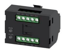
Electronics module IO-Link for ID key-operated switch, freely-programmable electronic switches, controller and RFID authentication of the switching function, black, operating voltage 24 V DC, screw terminal, for front plate mounting, for industrial application in control cabinets and machines
