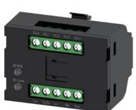
Electronics module IO-Link for ID key-operated switch, with 5 pre-programmed electronic switches, controller and RFID authentication of the switching function, black, operating voltage 24 V DC, screw terminal, for front plate mounting, for industrial application in control cabinets and machines
