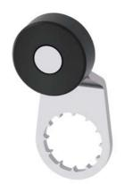
twist lever for position switch 3SE51 Stainless steel lever, Form A 27 mm long with plastic roller 19 mm functional at -40  $^{\circ}\text{C}$
