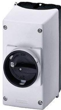
Molded-plastic enclosure for surface mounting Degree of protection IP55 with N and PE terminal Can be locked in O position 82 mm with metric cable gland No UL/CSA approval
