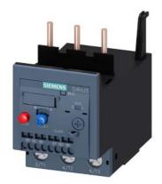
Overload relay 70...80 A Thermal For motor protection Size S2, Class 10A Contactor mounting Main circuit: Screw Auxiliary circuit: spring-type terminal Manual-Automatic-Reset
