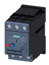
Overload relay 62...73 A Thermal For motor protection Size S2, Class 10A Standalone installation Main circuit: Screw Auxiliary circuit: spring-type terminal Manual-Automatic-Reset
