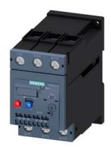
Overload relay 40... 50 A Thermal For motor protection Size S2, Class 10 Standalone installation Main circuit: Screw Auxiliary circuit: spring-type terminal Manual-Automatic-Reset
