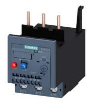
Overload relay 22...32 A Thermal For motor protection Size S2, Class 10 Contactor mounting Main circuit: Screw Auxiliary circuit: spring-type terminal Manual-Automatic-Reset
