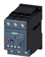
Overload relay 22...32 A Thermal For motor protection Size S2, Class 10 Standalone installation Main circuit: Screw Auxiliary circuit: Screw Manual-Automatic-Reset
