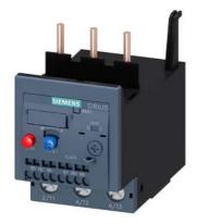
Overload relay 18...25 A Thermal For motor protection Size S2, Class 10 Contactor mounting Main circuit: Screw Auxiliary circuit: spring-type terminal Manual-Automatic-Reset
