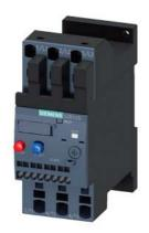
Overload relay 27...32 A Thermal For motor protection Size S0, Class 10 Standalone installation Main circuit: Spring-type terminal Auxiliary circuit: spring-type terminal Manual-Automatic-Reset
