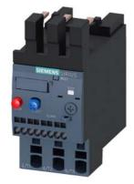
Overload relay 27...32 A Thermal For motor protection Size S0, Class 10 Contactor mounting Main circuit: Spring-type terminal Auxiliary circuit: spring-type terminal Manual-Automatic-Reset
