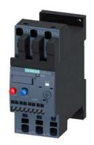
Overload relay 20...25 A Thermal For motor protection Size S0, Class 10 Standalone installation Main circuit: Spring-type terminal Auxiliary circuit: spring-type terminal Manual-Automatic-Reset
