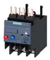
Overload relay 11...16 A Thermal For motor protection Size S0, Class 10 Contactor mounting Main circuit: Ring cable lug Auxiliary circuit: ring cable lug Manual-Automatic-Reset
