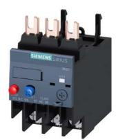
Overload relay 9.0...12.5 A Thermal For motor protection Size S0, Class 10 Contactor mounting Main circuit: Ring cable lug Auxiliary circuit: ring cable lug Manual-Automatic-Reset
