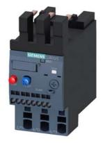
Overload relay 2.8...4.0 A Thermal For motor protection Size S0, Class 10 Contactor mounting Main circuit: Spring-type terminal Auxiliary circuit: spring-type terminal Manual-Automatic-Reset
