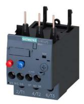
Overload relay 1.8...2.5 A Thermal For motor protection Size S0, Class 10 Contactor mounting Main circuit: Screw Auxiliary circuit: Screw Manual-Automatic-Reset
