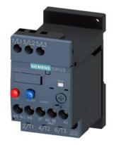
Overload relay 3.5...5.0 A Thermal For motor protection Size S00, Class 10 Standalone installation Main circuit: Screw Auxiliary circuit: Screw Manual-Automatic-Reset
