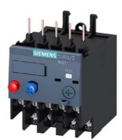
Overload relay 2.2...3.2 A Thermal For motor protection Size S00, Class 10 Contactor mounting Main circuit: Ring cable lug Auxiliary circuit: ring cable lug Manual-Automatic-Reset
