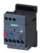
Overload relay 2.2...3.2 A Thermal For motor protection Size S00, Class 10 Standalone installation Main circuit: Screw Auxiliary circuit: Screw Manual-Automatic-Reset
