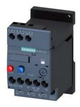
Overload relay 0.55...0.80 A Thermal For motor protection Size S00, Class 10 Stand-alone installation Main circuit: Screw Auxiliary circuit: Screw Manual-Automatic-Reset
