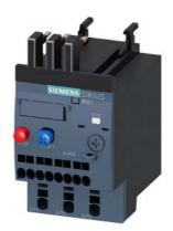
Overload relay 0.45...0.63 A Thermal For motor protection Size S00, Class 10 Contactor mounting Main circuit: Spring-type terminal Auxiliary circuit: spring-type terminal Manual-Automatic-Reset
