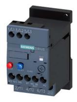
Overload relay 0.28...0.40 A Thermal For motor protection Size S00, Class 10 Stand-alone installation Main circuit: Screw Auxiliary circuit: Screw Manual-Automatic-Reset
