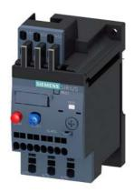
Overload relay 0.18...0.25 A Thermal For motor protection Size S00, Class 10 Stand-alone installation Main circuit: Spring-type terminal Auxiliary circuit: spring-type terminal Manual-Automatic-Reset
