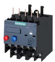
Overload relay 0.11...0.16 A Thermal For motor protection Size S00, Class 10 Contactor mounting Main circuit: Ring cable lug Auxiliary circuit: ring cable lug Manual-Automatic-Reset
