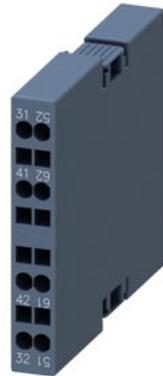
auxiliary switch, lateral, 2 NC, on the left: 51/52, 61/62, on the right: 31/32, 41/42, current path: 1 NC, 1 NC, spring-loaded terminal, for contactors 3RT2 and contactor relays 3RH2
