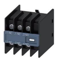
auxiliary switch, on the front, 1 NO + 2 NC, .1/.2, .1/.2, .3/.4, --/--, current path: 1 NC, 1 NC, 1 NO, --, ring cable lug connection, for contactors 3RT2 and contactor relays 3RH2
