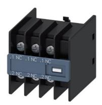
auxiliary switch, on the front, 3 NC, .1/.2, .1/.2, .1/.2, --/--, current path: 1 NC, 1 NC, 1 NC, --, ring cable lug connection, for contactors 3RT2 and contactor relays 3RH2
