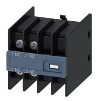
auxiliary switch, on the front, 2 NC, .1/.2, .1/.2, --/--, current path: 1 NC, 1 NC, --, --, ring cable lug connection, for contactors 3RT2 and contactor relays 3RH2
