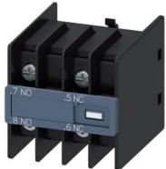
auxiliary switch, on the front, 1 NO + 1 NC, 11 U, .7/.8, --/--, .5/.6, --/--, current path: 1 NO (leading), --, 1 NC (lagging), --, ring cable lug connection, for contactors 3RT2 and contactor relays 3RH2
