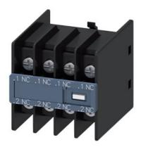
auxiliary switch, on the front, 4 NC, .1/.2, .1/.2, .1/.2, .1/.2, current path: 1 NC, 1 NC, 1 NC, 1 NC, ring cable lug connection, for contactors 3RT2 and contactor relays 3RH2
