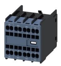
auxiliary switch, solid-state compatible, on the front, 2 NO + 2 NC, .1/.2, .3/.4, .3/.4, .1/.2, current path: 1 NC (solid-state compatible), 1 NO, 1 NO, 1 NC (solid-state compatible), spring-loaded terminal, for contactors 3RT2 and contactor relays 3RH2
