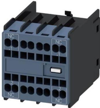
auxiliary switch, solid-state compatible, on the front, 2 NC, .1/2, --/--, --/--, .1/2, current path: 1 NC (solid-state compatible), --, --, 1 NC (solid-state compatible), spring-loaded terminal, for contactors 3RT2 and contactor relays 3RH2
