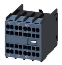
auxiliary switch, on the front, 3 NO, .3/.4, .3/.4, .3/.4, --/--, current path: 1 NO, 1 NO, 1 NO, --, spring-loaded terminal, for contactors 3RT2 and contactor relays 3RH2
