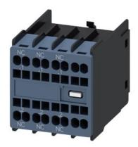
auxiliary switch, on the front, 3 NC, .1/.2, .1/.2, .1/.2, .-/--, current path: 1 NC, 1 NC, 1 NC, --, spring-loaded terminal, for contactors 3RT2 and contactor relays 3RH2
