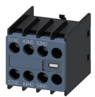
auxiliary switch, on the front, 2 NO + 1 NC, 31/32, 43/44, 53/54, --/--, current path 1 NC, 1 NO, 1 NO, --, screw terminal, for contactors 3RT2 and contactor relays 3RH2
