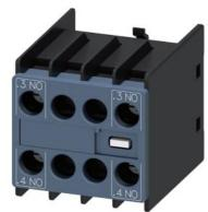
auxiliary switch, solid-state compatible, on the front, 2 NO, .3/.4, --/--, .3/.4, current path: 1 NO (solid-state compatible), --, --, 1 NO (solid-state compatible), screw terminal, for contactors 3RT2 and contactor relays 3RH2
