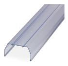
Cover profile for covering terminal strips, snaps onto AP 3-TU, AP 3-TNS 35 cover profile carriers, can be labeled with AP-ES insert strip. A cover profile carrier is to be positioned at the ends and at intervals of around approx. 40 cm. Supply length: As per customer order
