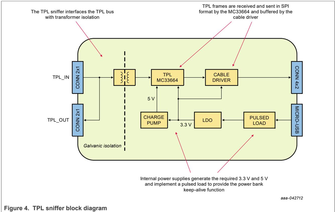
Figure 4. TPL sniffer block diagram
