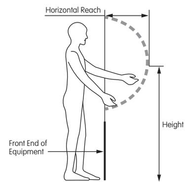
The table and illustration show the mounting range for the assembled emergency stop switch and protective guard. The height and horizontal reach are determined according to SEMI S8.
