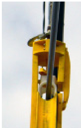
Cable Capture Prevents Pull Tape Or Cable Jumping Edge
