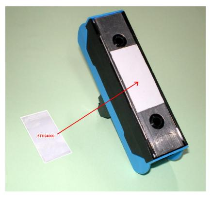
These thermal PAD with very good thermal conduction have also an electrical conduction. So all the mechanical parts stay connected to the earth. With some silicone thermal PAD the earth conduction is not achieved
