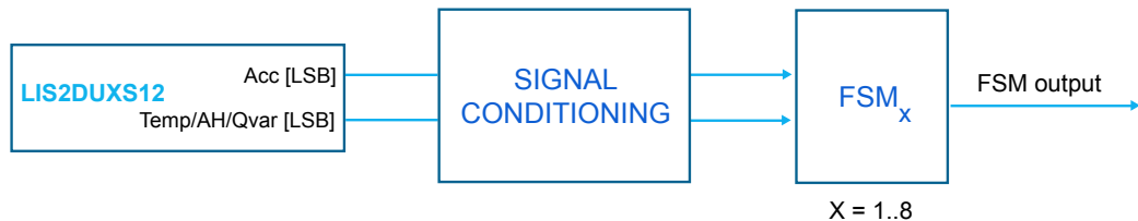
Figure 12. State machine in the LIS2DUXS12
