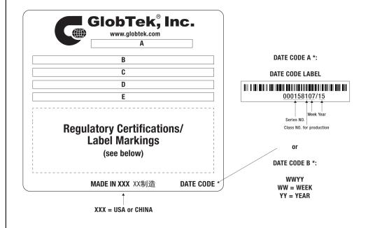
A=ICT / ITE / Medical Power Supply B=P/N: (料号) WR97A2000CCPMFR6B C=Model (型号) GTM86100-1005-W2A D=Input (输入)100-240V~, 50-60Hz, 0.3A E=Output (输出)5.0 V == 2.0 A, 10.00W
