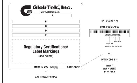
A=ICT / ITE / Medical Power Supply B=P/N: (料号) TR9KX2222LCP-IM(R6B) C=Model (型号) GTM961200P12054-T2 D=Input (输入)100-240V~, 50-60 Hz, 1.5 A E=Output (输出)54.0 V == 2.22 A, 120.00W
