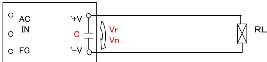
Vr : Measure point of line/load regulation and output voltage.
