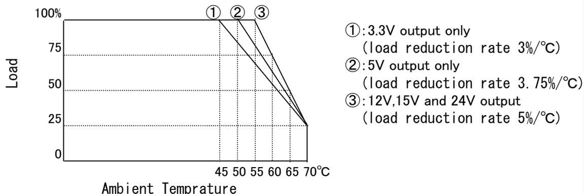
Note) 3.3V and 5V outputs are the input voltages of 100V or less and output current Dirating of 1%/V is necessary.
