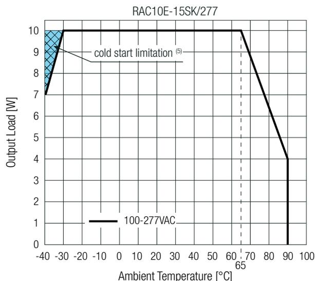
Note5: Cold start is limited to reduced output Power for 15V in general and for 3.3 to 12V versions at use in low line conditions
