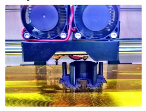
The build surface needs to be level to ensure the filament properly sticks to the surface and to provide a secure foundation for the print job. The bed can be leveled by either mechanically leveling the bed or using a raft to accommodate for unevenness.
