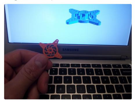
In order to produce 3D printer compatible objects, it is important to understand its limits. I like to think of a 3D printer as a spaghetti machine. It carefully stacks noodles on top of each other, and if there isn't enough noodle to stack on, it droops. The
