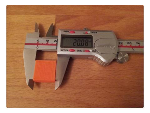
Scale calibration illustrates the process in which you compare the desired dimensions with the actual dimensions your printer produces. The easiest method for accomplishing this is to start by printing a calibration object, like a <a href="Calibration">Calibration</a> (https://adafru.it/cos) or the <a href="Calibration Vector">Calibration Vector</a> (https://adafru.it/cot). Once complete, use a set of calipers to check the dimensions and record your results.
