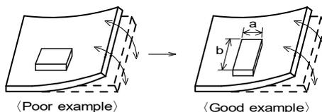
(2) Components location on PCB separation
